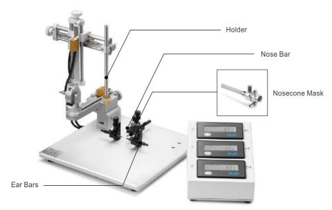
Portable Mouse Srereotaxic Instrument
